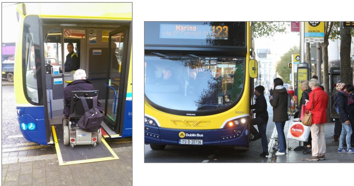
Figure 5.12 Having buses flush with the bus stop is important to allow the ramp to lower correctly, but also to speed up the boarding and alighting of all passengers as gaps slow this down.
